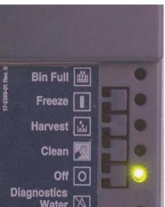
**To Test**: Move the float stick slowly up and down and observe the light display on the controller. **Results:**
